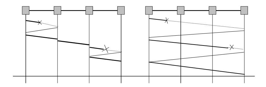
Link ARQ is faster than E2E ARQ when there are many errors
