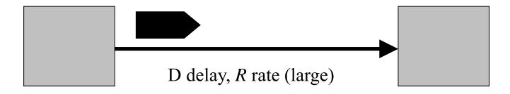
Large R (fast)  $\rightarrow$  small Tx Time (M/R) Ex: OC-3 (D = 10ms, R = 155Mb/s, M = 1KB) Tx Time = .010 + ((1024 × 8)/(155 × 1024 × 1024)) = 0.01005 sec = 10.05 ms (D >> M/R)
