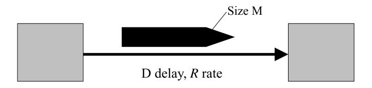
Tx delay = (M bits)/(R b/s) = M/R secProp delay = D sec = Length/Prop\_speed **Total Tx Time = D + M/R sec**
