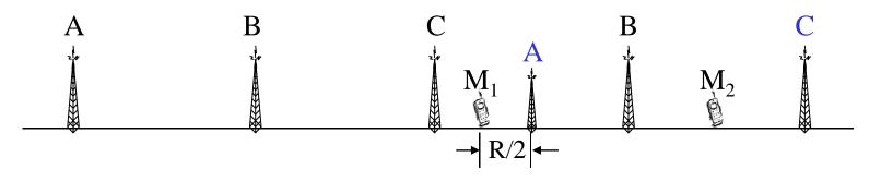
$$\begin{split} M_1 & \text{in the smaller cell A, in general, has better C/I} \\ C/I &= \{(9R/2)/(R/2)\}^4 = 9^4 > 5^4 \\ M_1 & \text{tx in low power} \\ M_2 & \text{in the larger cell C has worse C/I} \\ C/I &= (3R/R)^4 = 3^4 < 5^4 \\ M_2 & \text{tx in high power} \end{split}$$
