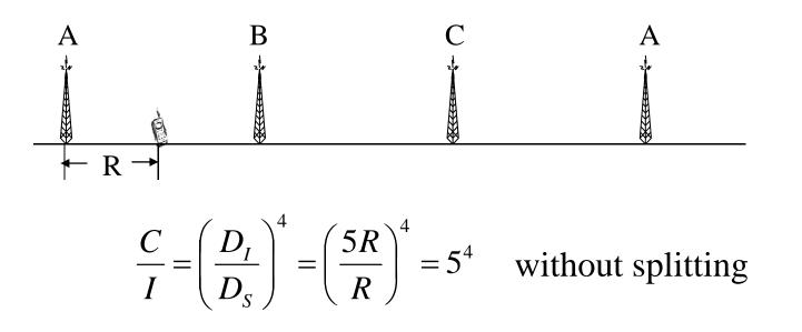
large cell + small cell due to traffic density
